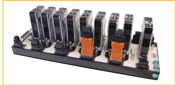
Figure 2. A fieldbus power conditioner prevents the high frequency communications signal from being shorted out by the DC voltage regulators. Typical power conditioners make 350 to 500mA available on the bus.
