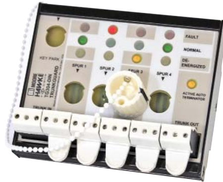
Figure 10. Device couplers with key-operated interlock permit fieldbus devices to be de-energized for “live” maintenance in Zone 1/Zone 2 without de-powering the entire segments.
