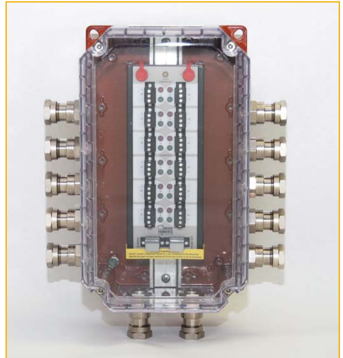
Figure 3. A device coupler provides short circuit protection on each spur. Some device couplers have automatic segment termination.
